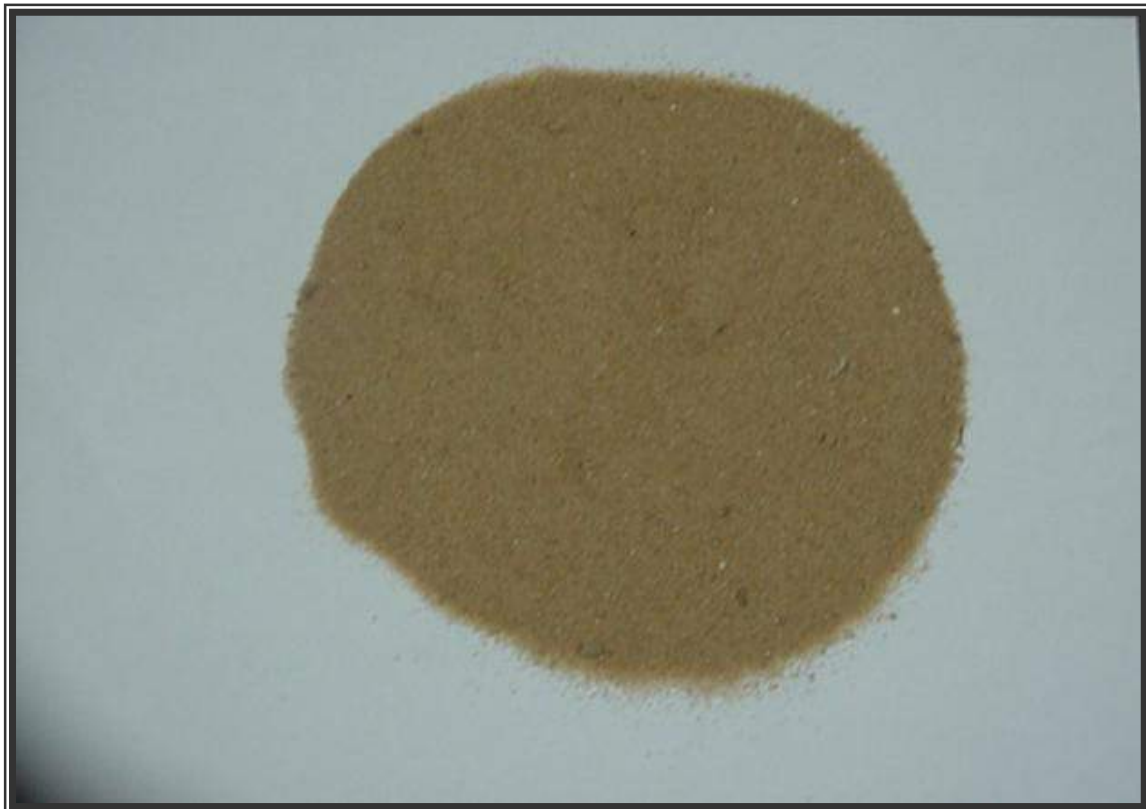
Fig (6.2) the Sand sample used in the experiment ( d_{50} = 0.3 mm)
