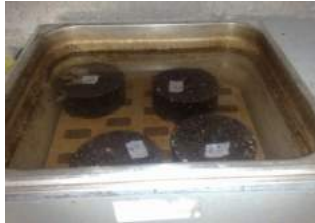
Figure (F.10): Water bath for Marshal Samples
