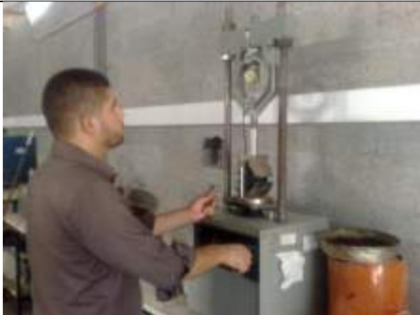
Figure (F.11): Testing Marshal Samples for stability and flow
