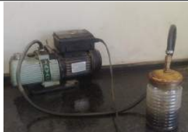
Figure (F.12): Measuring the theoretical density of asphalt mix using Pycnometer
