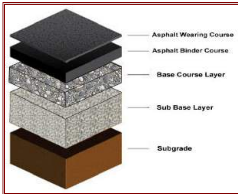
Figure (2.1): Flexible Pavement Layers
