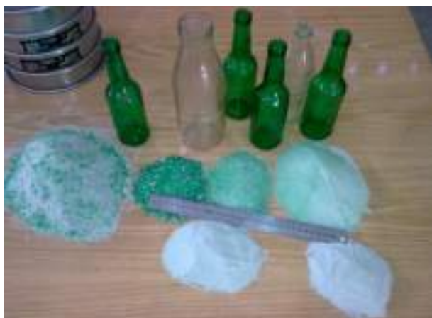
Figure (F.3): Waste glass sieve analysis
