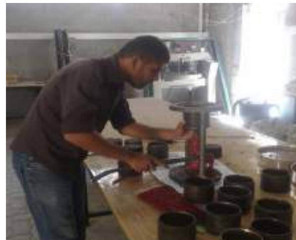
Figure (F.6): Removing Marshal samples molds after compaction
