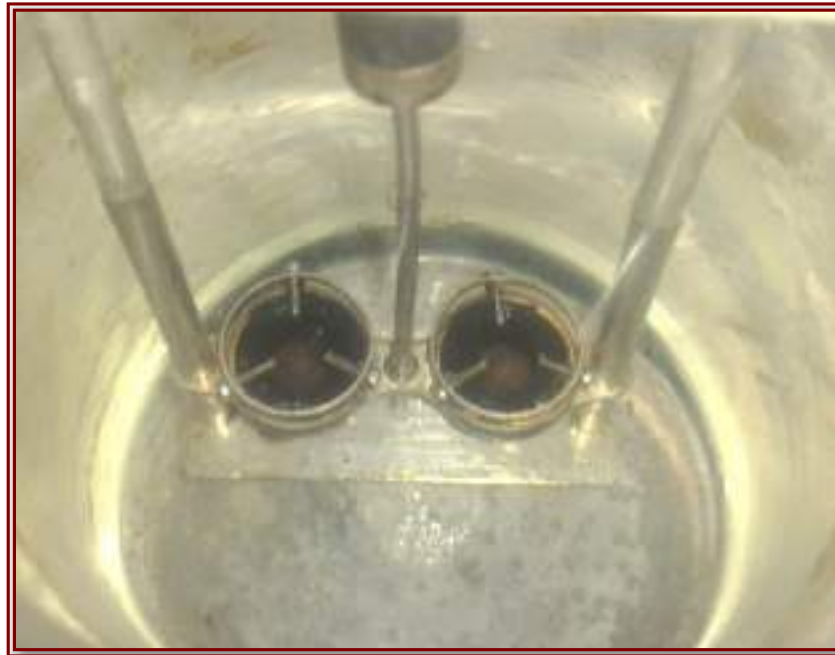
Figure (4.3): Softening point test for bitumen samples
