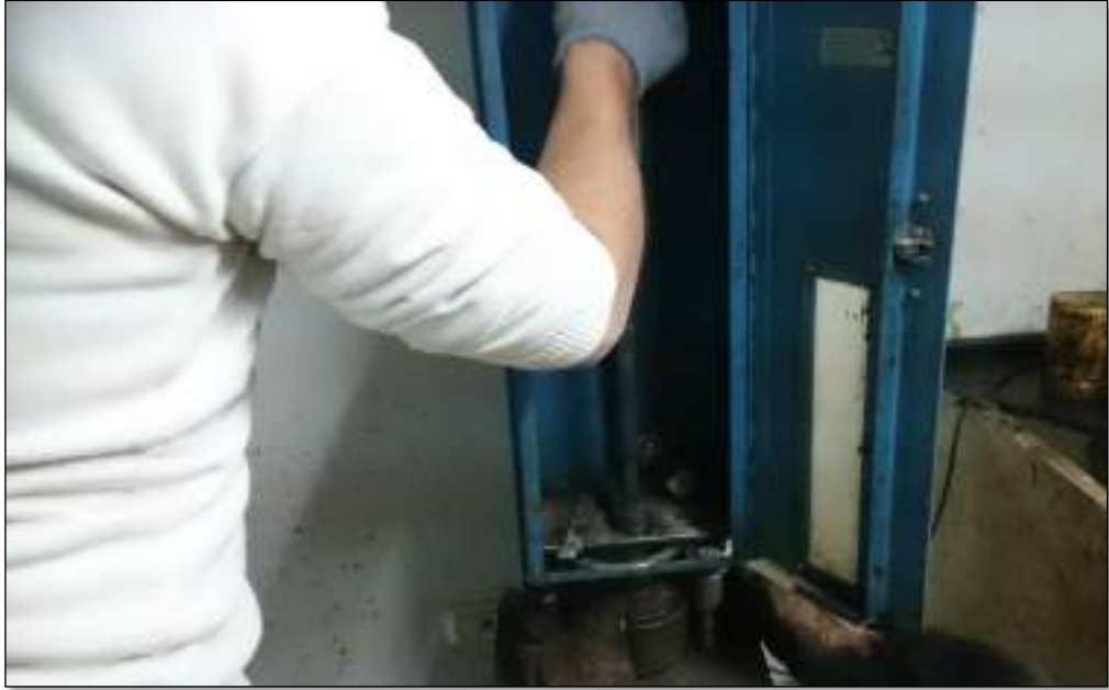
Figure 0E.7: Asphalt mix during compaction
