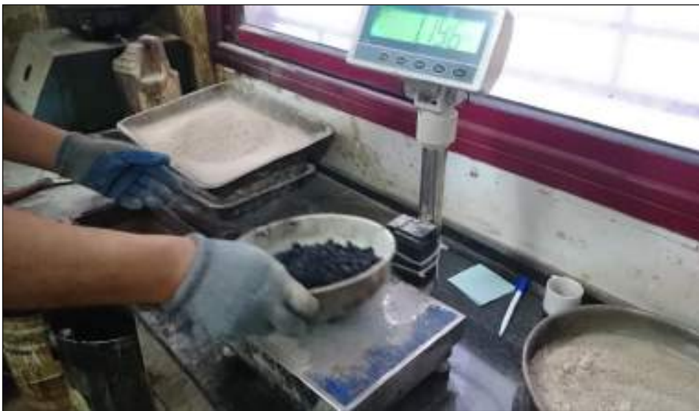
Figure E.4: preparing of marshal samples
